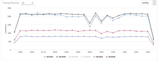
Any traffic flow in the graph represents a clear indication that the Falcon sensor for Windows is configured correctly to work with the domain controller. If there is no traffic flow, see
